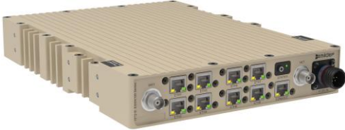
C3354 – Switch with 1G ports, WiFi and 5G.
