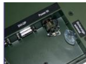
RD19 with circuit breaker
