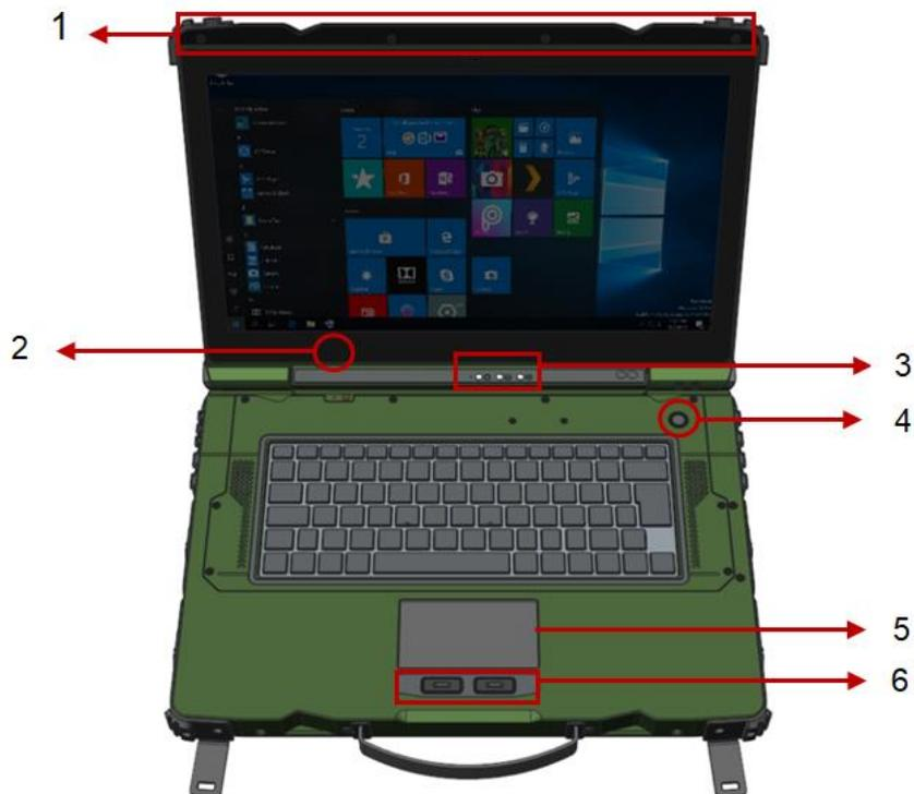
1. Embedded Antennas (Optional): GPS, WLAN/ BT x 2
