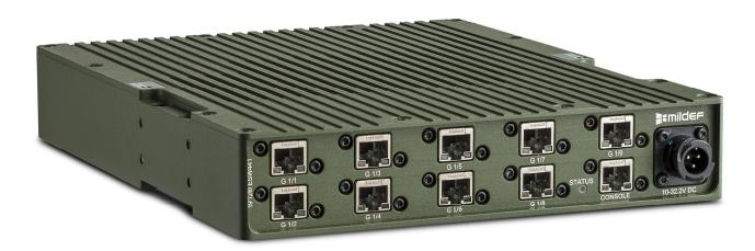
The 19"/2® 17-port Switch ESW442 is a powerful managed switch which features dual 1 Gbps fiber uplinks and fifteen 1 Gbps access ports. An ideal solution for demanding high speed networks, including data, video, and voice services. It supports both layer 2 and layer 3 functionality and can be implemented anywhere high speed LAN and WAN connectivity may be required.
