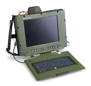
MilDef DR Keyboard KBD211 for use together with Panther DR-series. When it's not used it serves as a screen protector for the Panther as it can be folded over the screen. It can also easily be removed from the Panther and used together with other computers as it has a standard USB interface.
