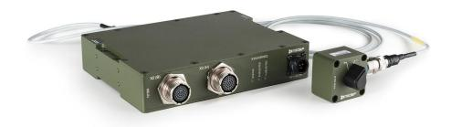
The KSW502 is a KVM switch for DVI and USB in a fully rugged enclosure. It allows 2 computers to share the use of a single monitor via DVI and keyboard/mouse via 2x USB. The peripheral focus will be given to a computer manually by using the external switch.
