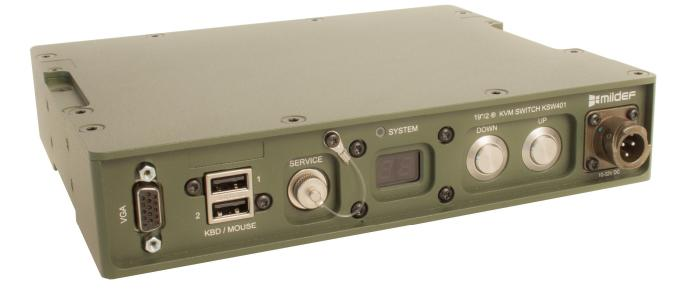
The KSW401 is a KVM switch for VGA and USB input in a fully rugged enclosure. It allows up to 7 computers to share the use of a single VGA and 2x USB for keyboard and mouse.
